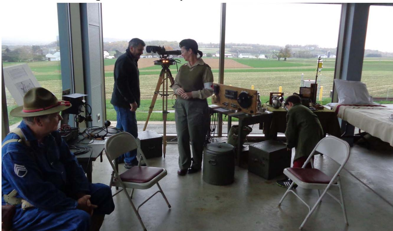
Another view of the fire control and communications display shows the BD-71 switchboard in the center and two EE-91 telephones on the far right of the picture on a table. All telephones are connected to the switchboard and can communicate together.
